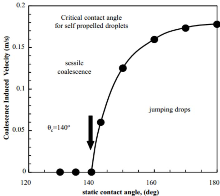
Fig. 6. Effects of the static contact angle on the droplet jumping speed, and determination of critical contact angle for jumping phenomenon ( $\theta_c = 140^\circ$ )
